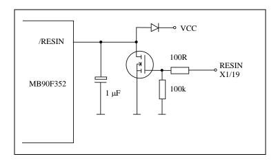
Figure 4: structure of /RESIN Line
