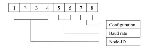
Figure 2: DIP-switch Pinout and Functions
