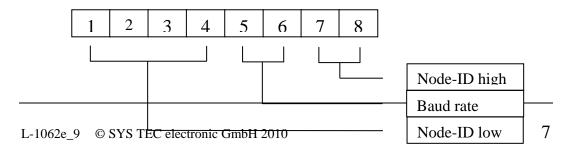
Figure 3: DIP-switch Pinout and Functions, version 3301002 only
