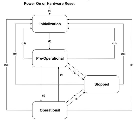
Figure 5: State Diagram of a CANopen Device
